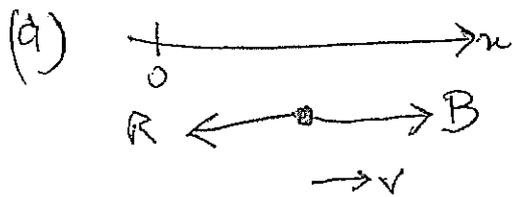
$$\begin{aligned} \text{Nett force} &= B - R \\ &= 410 - 50 \\ &= 360 \text{ N} \end{aligned}$$
